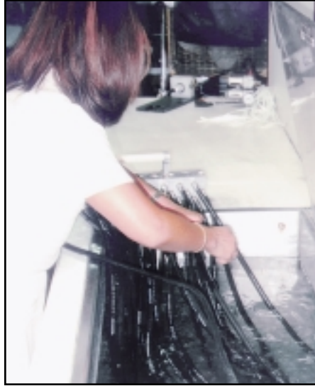
Testing is conducted on the hose assemblies prior to final production.
