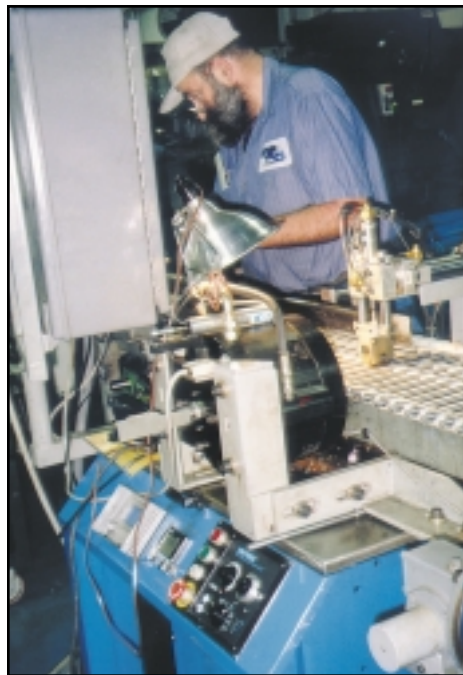
M. K. Chambers automated the Finn-Power CC20 crimper with a table. Washers and lead screws are put on the walking beam table. It automatically feeds it into the Finn-Power CC20 for crimping.
