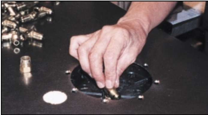
Stem section is inserted into the nut.
