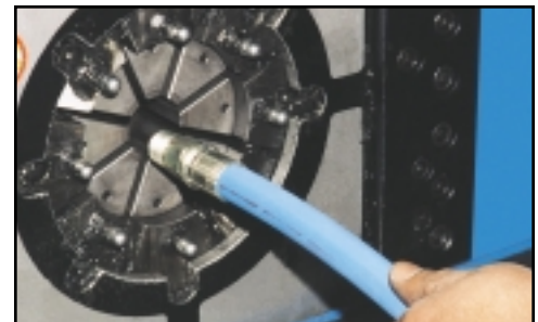
The FP120 crimps to an exact dimension and can adjust in .01 mm increments. To ensure speed and accuracy on all jobs,
