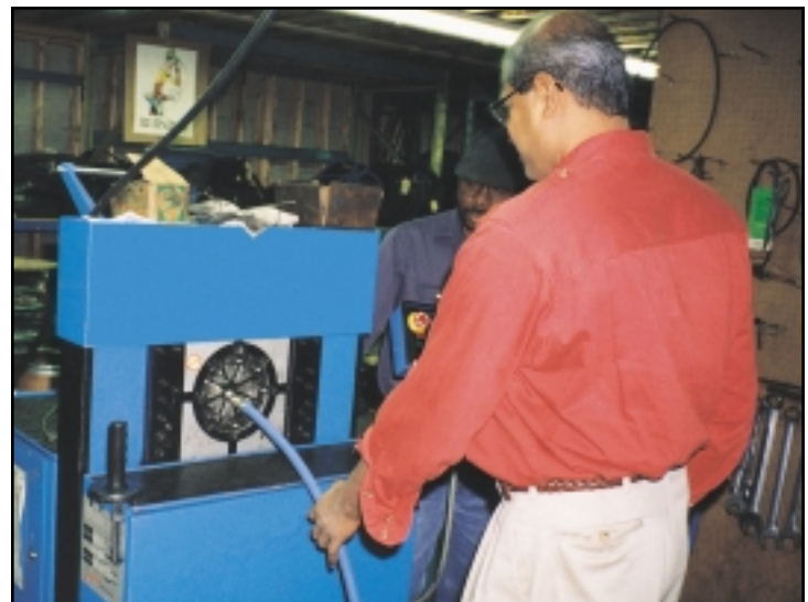
The FP120 crimps to an exact dimension and can adjust in .01 mm increments. To ensure speed and accuracy on all jobs,
