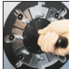
The head is closed and the dies are engaged by master die sets.
