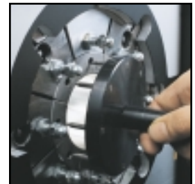
The tool is removed and the swaging machine is ready for operation.
