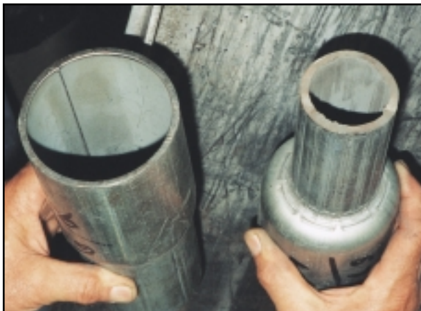
The Finn-Power P32 swaging machine gives Sunguard Shade Structures the flexibility of design to make a larger or smaller pipe fit into the same size superstructure pieces simply by changing the dies. Example: A 4" O.D. pipe can be reduced to 2.875" OD."
